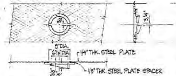
READING-HOLE COVER FRAME DETAIL NOT TO SCALE
