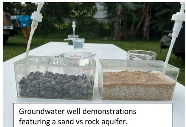
Groundwater well demonstrations featuring a sand vs rock aquifer.
