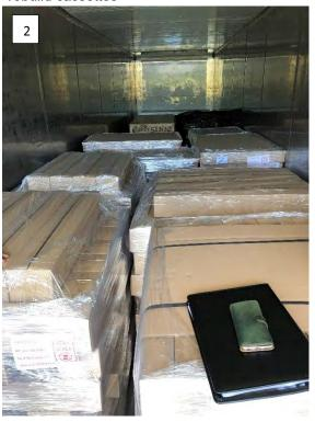
[3 & 4] 11 frames of membrane modules stored in a container in a shaded area to regulate the temperature
